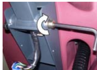
Insert handle assembly in between bushings. Insert the shoulder bolt through the bushing and screw into the handle assembly using supplied wrench.
