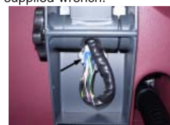
The wire harness must be aligned with the patterns on the connector to fit.
