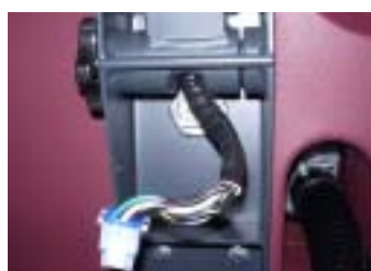
Attach the wire harness to the machine.
